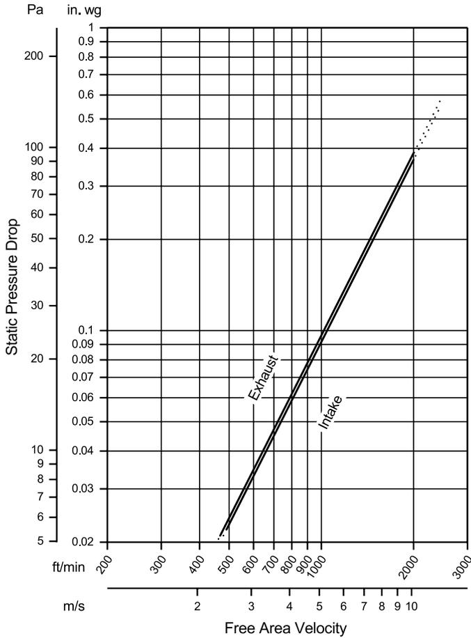
Model AFJ-120 resistance to airflow (pressure drop) varies depending on louver application (air intake or air exhaust). Free area velocities (shown) are higher than average velocity through the overall louver size. See louver selection information. (Test Figure 5.5-6.5)
