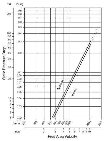
Model AFA-801 resistance to airflow (pressure drop) varies depending on louver application (air intake or air exhaust). Free area velocities (shown) are higher than average velocity through the overall louver size. See louver selection information. (Test Figure 5.5-6.5)
