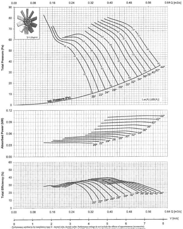
Performance certified is for installation type D - ducted inlet, ducted outlet. Performance ratings do not include the effects of appurtenances (accessories).
