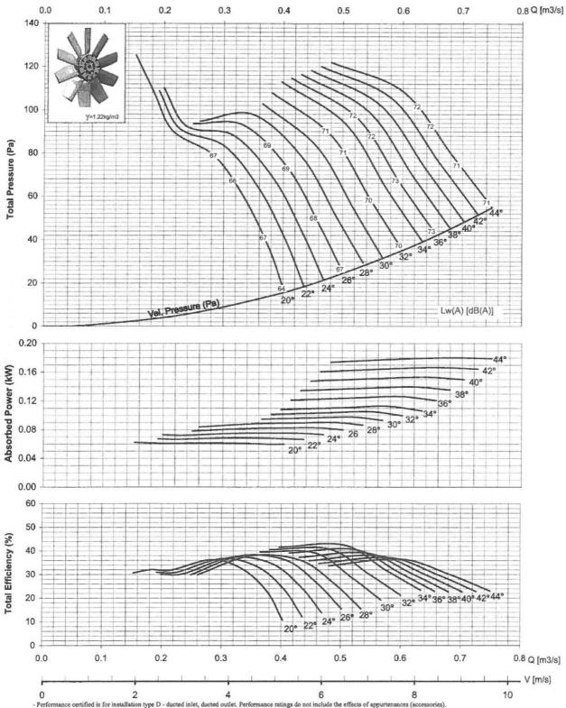
Performance certified is for installation type D - ducted inlet, ducted outlet. Performance ratings do not include the effects of appurtenances (accessories).
