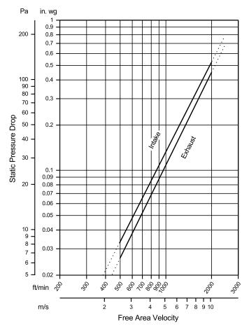
Model EAD-401 resistance to airflow (pressure drop) varies depending on louver application (air intake or air exhaust). Free area velocities (shown) are higher than average velocity through the overall louver size. See louver selection information. (Test Figure 5.5-6.5)
