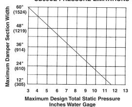
The CD50CE may be used in systems with total pressures exceeding 3.5" by reducing damper section width as indicated. Example: Maximum design total pressure of 8.5" w.g. would require CD50CE damper with maximum section width of 36" (914).
