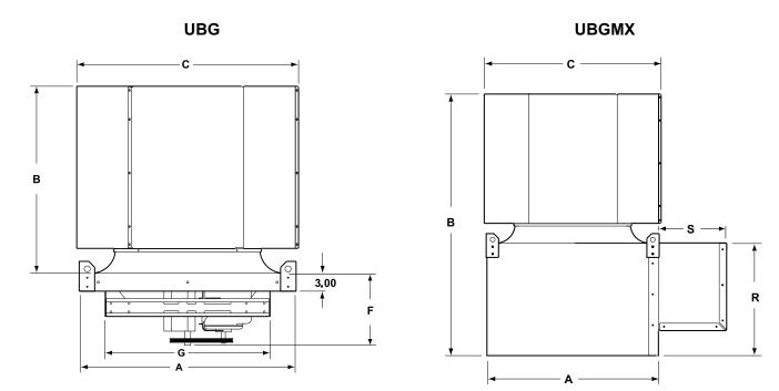
Typical drawings are for dimensional purposes only which are correct within limits suitable for normal installation requirements and do not necessarily show actual construction. All dimensions are in inches.
