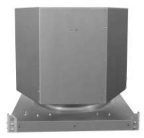
Model UBG low silhouette belt drive exhausters are ideally suited for moving large volumes of air. Capacities range from 3,770 to 83,370 CFM and up to <sup>3</sup>/<sub>4</sub> inch static pressure. The UBG is a high velocity exhauster design to discharge air up and away from the building. Typical applications includes all types of commercial and industrial facilities such as warehouses, foundries, mills and manufacturing plants.
