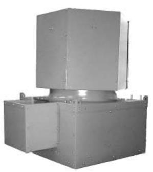
UBGMX exhausters with UF and SE options are designed and constructed to remove high temperature exhaust and smoke. These specially equipped ventilators meet IRI (Industrial Risk Insurers) requirements for exhausting 500 F air for 4 hours and SBCCI's "Standard Fire Prevention Code" requirements for exhausting 1000 F air for 15 minutes. The Butterfly Damper on the SE option meets the requirements of UL 793 for automatically opening under snow or dust load in an emergency situation.
