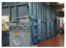
Air Test Chamber Greenheck has on-site registered air performance test chambers to measure air volume and horsepower requirements at different pressure levels.
