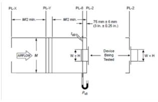
AMCA Standard 500-D (leakage), figure 5.4 Alternate.
