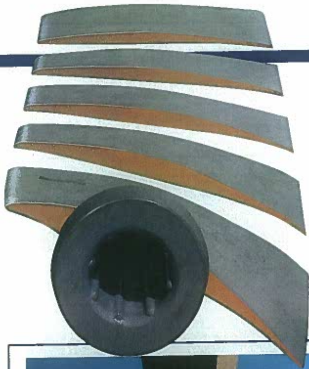
Airfoil Cross-Sections Gradually Increase From Tip to Root
