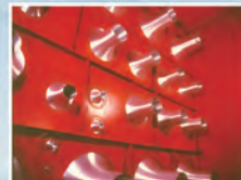
流量噴嘴 Multiple Nozzles for Flow Measurement
