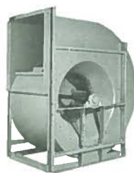
ARRANGEMENT 3, SISW For belt drive. Wheel centering between bearings. For industrial applications, ventilation and air conditioning.
