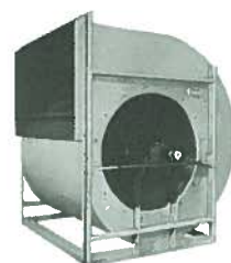
ARRANGEMENT 3, DIDW For belt drive. Similar to Arrangement 3, single width construction and application. For large volumes of air.
