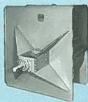
ARRANGEMENT 1, SISW For belt drive, open inlet. Wheel overhung. For elevated temperatures, corrosive fumes or ventilation and air conditioning applications.
