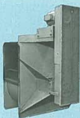
ARRANGEMENT 9, SISW For belt drive similar to Arrangement 1 except for provision to mount motor on top or side of fan.
