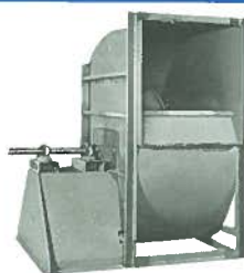
ARRANGEMENT 1, SISW For belt drive, open inlet. Wheel overhung. For elevated temperatures, corrosive fumes or ventilation and air conditioning applications.
