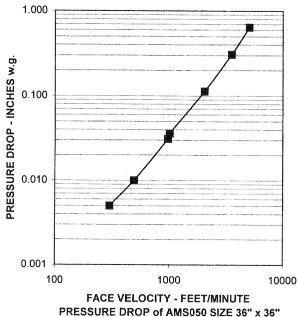
Ruskin Company certifies that the AMS050 Air Monitoring Station shown herein is licensed to bear the AMCA Certified Rating Seal - Airflow Measuring Station Performance. The ratings shown are based on tests and procedures performed in accordance with AMCA publication 611 and comply with requirements of the AMCA Certified Ratings Program. The AMCA Certified Ratings Seal applies to airflow measurement performance only.
