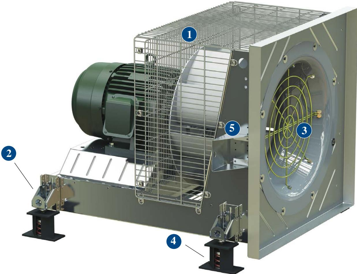
**1 Protective Enclosure** Grill style protective enclosure completely encloses all sides and the back of the fan wheel to protect personnel from moving fan parts. The panels are individually removable to provide access to the wheel for service or inspection. Enclosures are available with or without a panel to enclose the bottom of the fan. Protective enclosures are plated wire.
