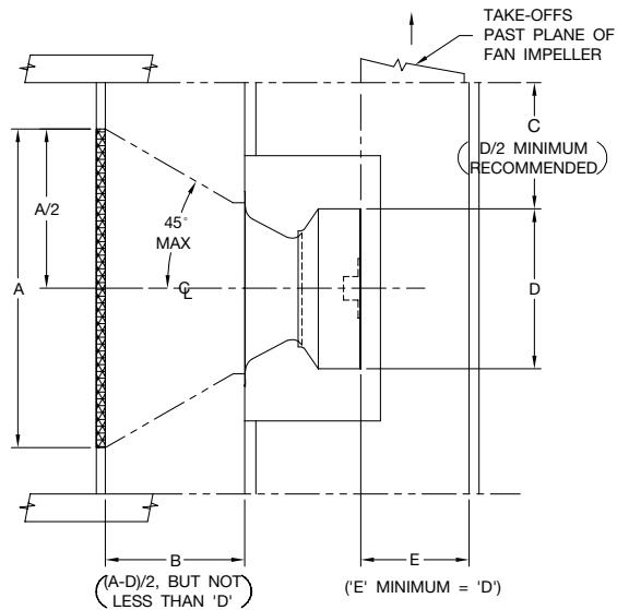
Figure 2. Flow Baffle and Vortex Spin Breaker Location
