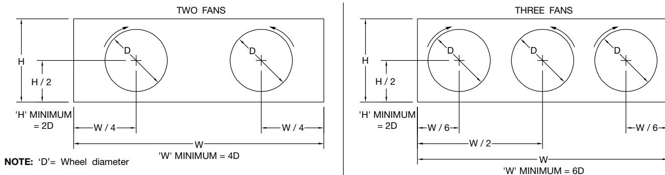
Figure 1. Recommended Location of Fan in Plenum
