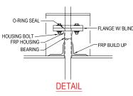
MODEL 204 HAS A SHAFT SEAL. MODEL 204 IS DESIGNED FOR ISOLATION SERVICE.
