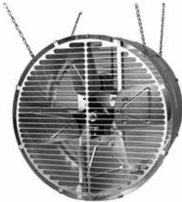
Type FH Horizontal Air Fans feature heavy gauge galvanized steel motor mounts, fan guards, and fan casing to provide the durability and corrosion resistance needed for greenhouse environments. Each FH fan comes with a chain mounting kit.
