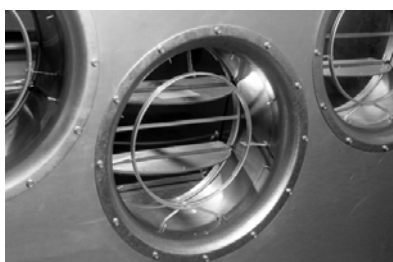
Figure 10. Piezometer ring measures inlet air flow.
