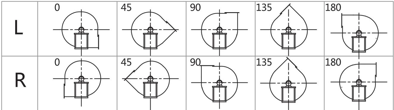
The rotation is identified from the view of the motor side. The rotation must be specified before placing orders; otherwise, the undesired rotation may cause installation problems.
