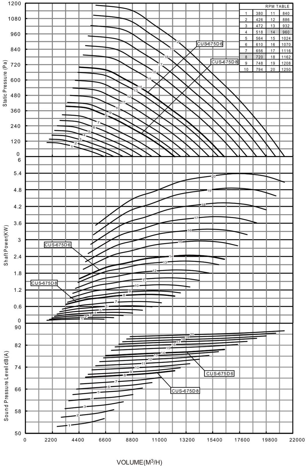
Performance certified is for installation type B - free inlet, ducted outlet. Power rating (kW) does not include transmission losses. Performance ratings do not include the effects of appurtenances (accessories). dB(A) A-weighted sound pressure level is based on 11.5 dB sound attenuation per octave band at 1.5m. Note that dB(A) levels are not licensed by AMCA International.
