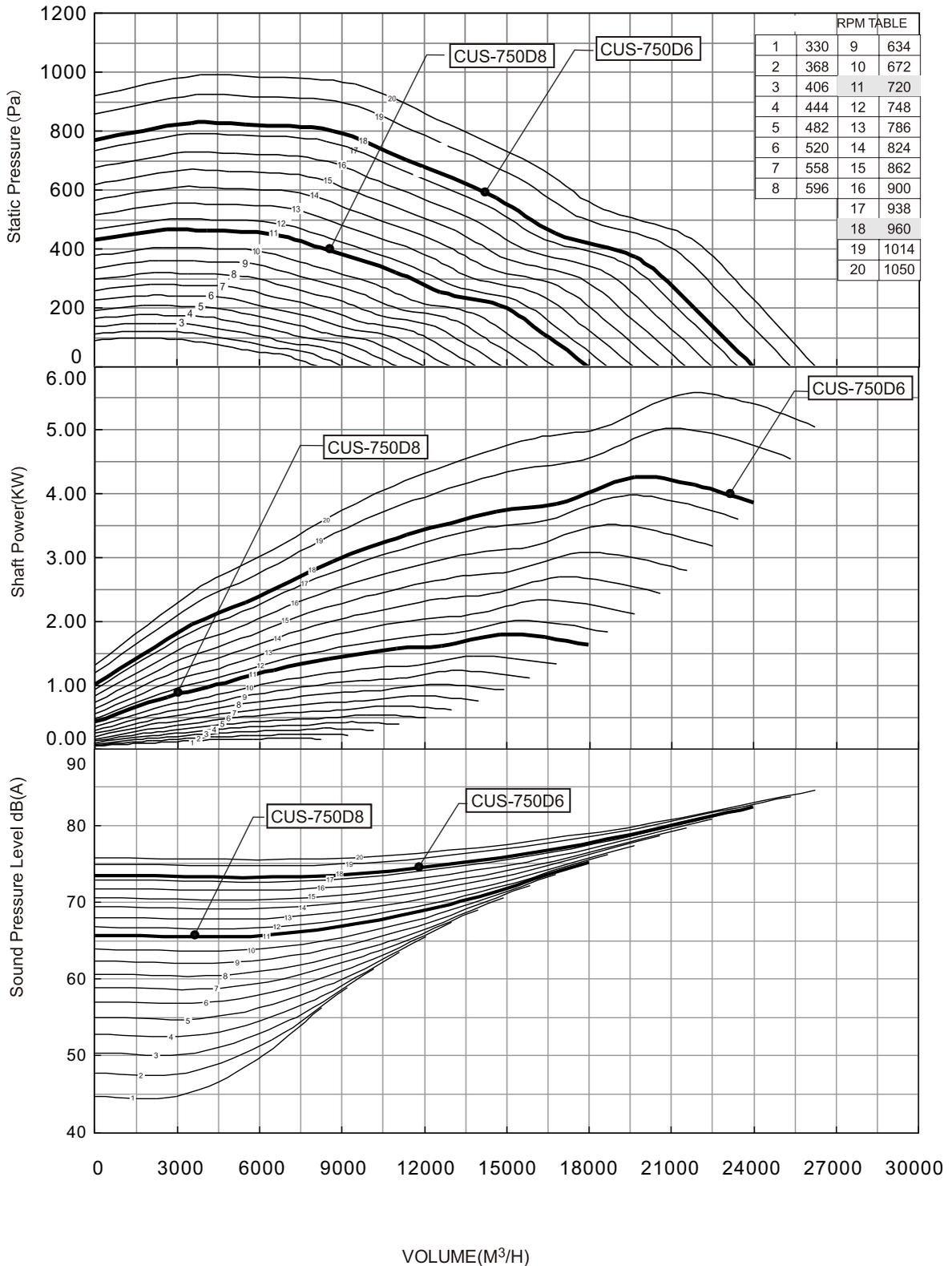
Performance certified is for installation type B - free inlet, ducted outlet. Power rating (kW) does not include transmission losses. Performance ratings do not include the effects of appurtenances (accessories). dB(A) A-weighted sound pressure level is based on 11.5 dB sound attenuation per octave band at 1.5m. Note that dB(A) levels are not licensed by AMCA International.
