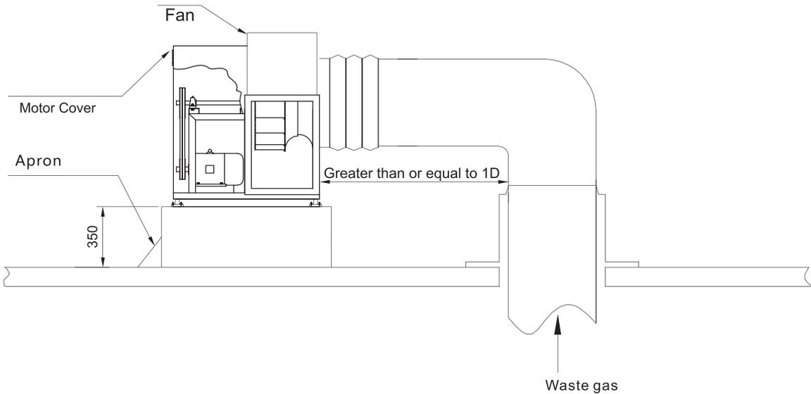
CUS fans are suitable for exhausting kitchen fumes in hotels. Before installation, the fans must be checked and cleaned to ensure the free rotation of the wheel. The fans shall not interfere with each other and can be well maintained. There shall be enough space left for removing the wheel and bearing. Rain cover shall be chosen for outdoor installation to protect the electrical components.
