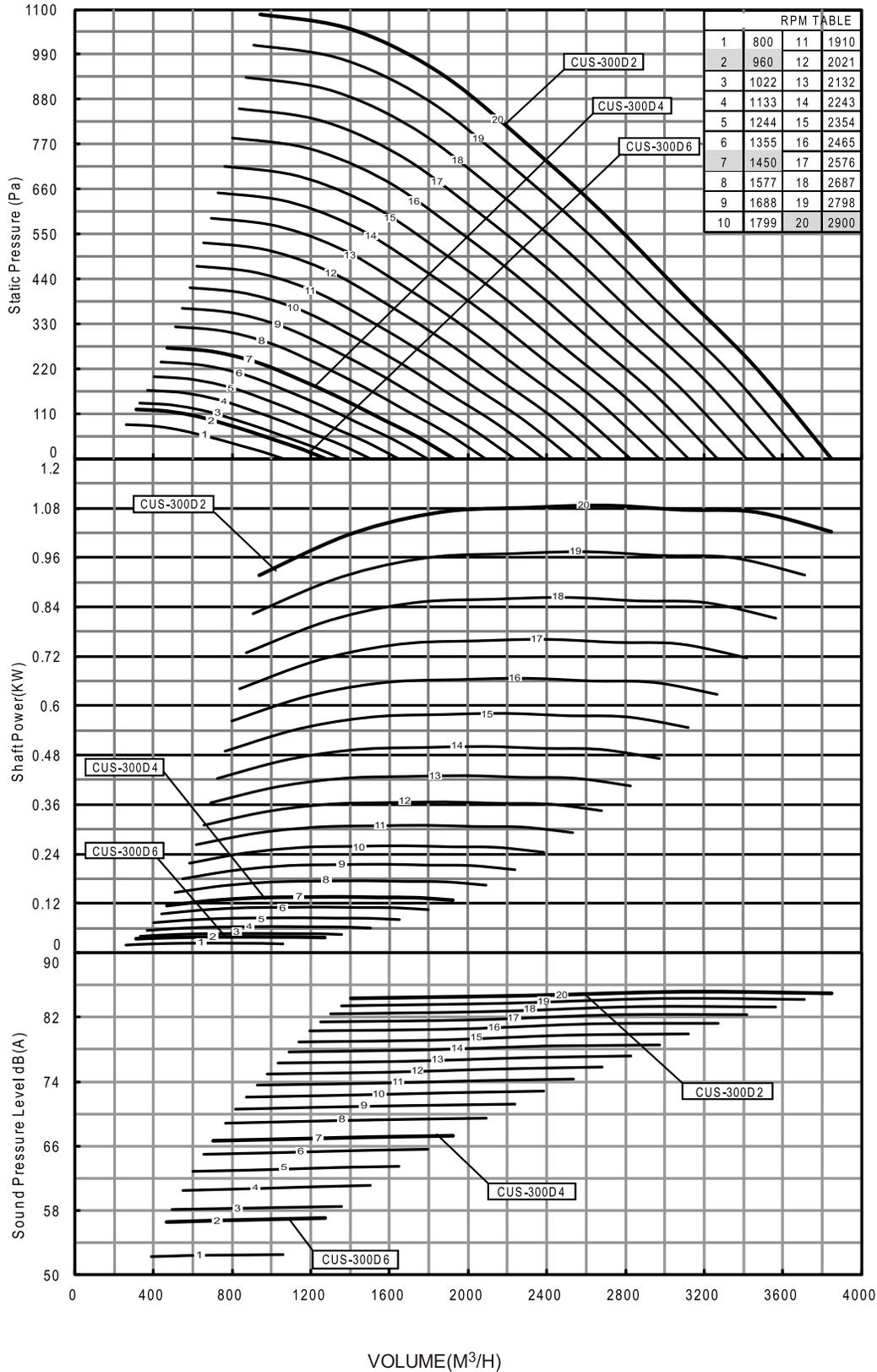
Performance certified is for installation type B - free inlet, ducted outlet. Power rating (kW) does not include transmission losses. Performance ratings do not include the effects of appurtenances (accessories). dB(A) A-weighted sound pressure level is based on 11.5 dB sound attenuation per octave band at 1.5m. Note that dB(A) levels are not licensed by AMCA International.
