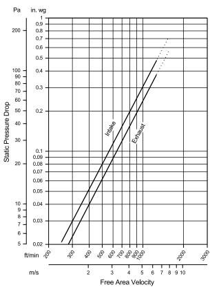
Model K605 resistance to airflow (pressure drop) varies depending on louver application (air intake or air exhaust). Free area velocities (shown) are higher than average velocity through the overall louver size. See louver selection information. (Test Figure 5.5-6.5)
