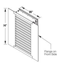
Non-Flanged \*Grille dimensions furnished approximately 1/2" (13) undersize Jamb Flange/ Internal Mount (single section wide only) \*Grille dimensions furnished approximately 1/2" (13) undersize
