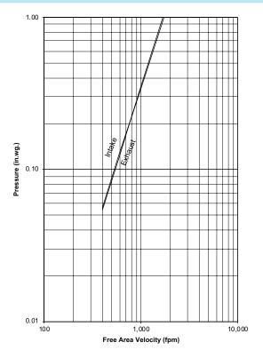
Louver Test Size =  $48" \times 48"$  (1219 × 1219) Pressure loss tested in accordance with Figure 5.5 of AMCA Standard 500-L. Data corrected to standard air density.
