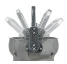
Designed to mount to any ceiling structure using the supplied steel mounting cable and Gripple® hanging hardware. Yoke mounting bracket allows for field-adjustment of hanging angle up to 45°.
