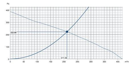
Performance certified is for installation type C - Ducted inlet, free outlet. Performance ratings do not include the effects of appurtenances (accessories).
