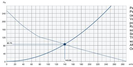
Performance certified is for installation type C – Ducted inlet, free outlet. Performance ratings do not include the effects of appurtenances (accessories).
