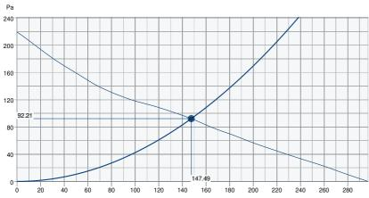
Performance certified is for installation type C – Ducted inlet, free outlet. Performance ratings do not include the effects of appurtenances (accessories).
