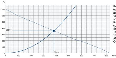
Performance certified is for installation type C – Ducted inlet, free outlet. Performance ratings do not include the effects of apputtenances (accessories)
