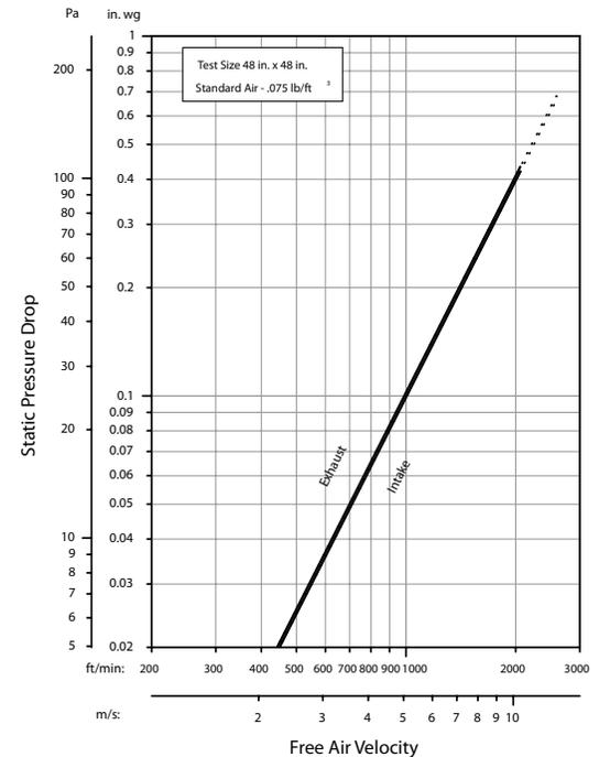
Louver Type T9106X resistance to airflow is shown with louver blades fully open. Resistance (pressure drop) varies depending on louver application (air intake or air exhaust). Free area velocities (shown) are higher than average velocity through the overall louver size. (Test Figure: 5.5-6.5)
