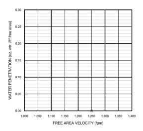
The AMCA Water Penetration Test provides a method for comparing various louver models and designs as to their efficiency in resisting the penetration of rainfall under specific laboratory test conditions. The point of zero water penetration is defined as that velocity where the water penetration curve projects through .01 oz of water penetration per sq. ft. of louver area. The beginning point of water penetration for RSR-550 is 1250 fpm free area velocity.
