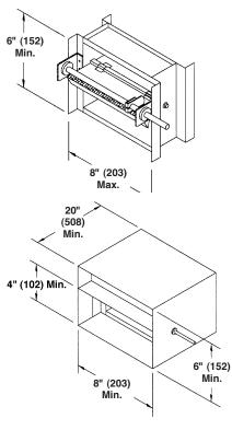
Nominal – 8"w x 6"h (203 x 152). Dampers with heights (B dimension) less than 8" (203) require Style B transitions and a sleeve. The damper itself remains 8" (203) high.
