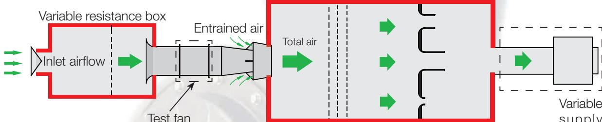
**AMCA 260 - Figure 1 - Test Setup**
