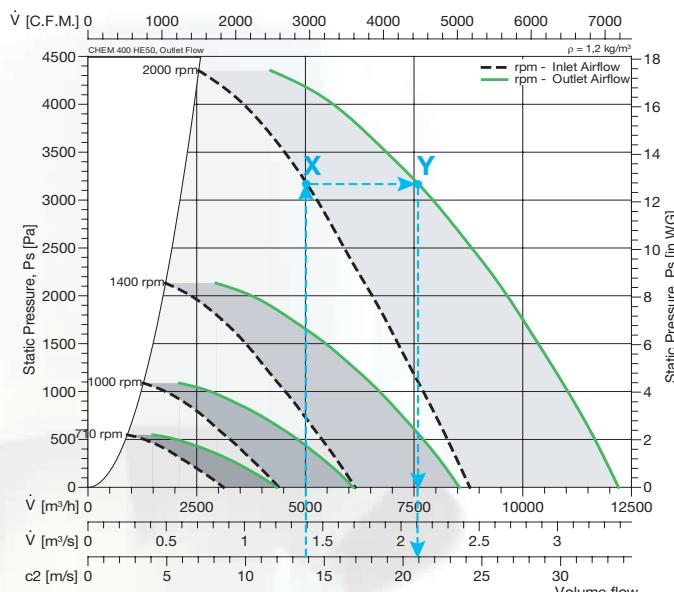
Figure 5, CHEM HE50 400 Outlet airflow curve
