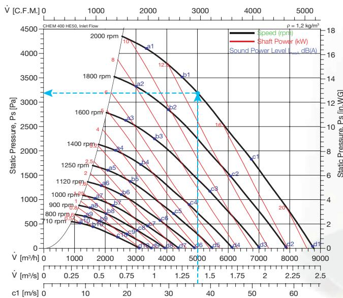
Figure 4, CHEM HE50 400 Inlet airflow curve
