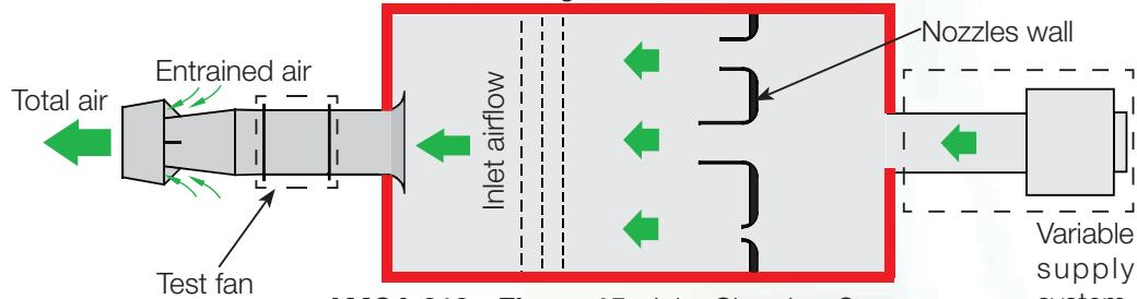
**AMCA 210 - Figure 15 - Inlet Chamber Setup**
