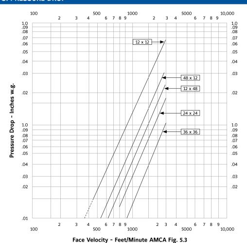
CD50 sizes 12 x 12, 24 x 24, 48 x 12, 12 x 48, 36 x 36 (305 x 305, 610 x 610, 1219 x 305, 305 x 1219, 914 x 914) All data corrected to represent standard air at a density of 0.075 lbs/ft<sup>3</sup>.
