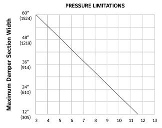
Maximum Design Total Static Pressure Inches Water Gage
