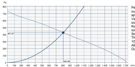
Performance certified is for installation type D-Ducted inlet, Ducted outlet. Performance ratings do not include the effects of appurtenances (accessories).
