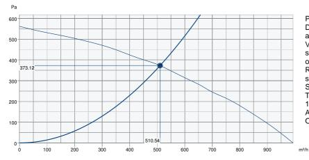
Performance certified is for installation type D – Ducted inlet, Ducted outlet. Performance ratings do not include the effects of appurtenances (accessories).
