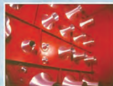
流量噴嘴 Multiple Nozzles for Flow Measurement
