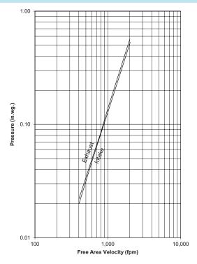
Louver Test Size = 48" x 48" (1219 x 1219) Pressure loss tested in accordance with Figure 5.5 of AMCA Standard 500-L. Data corrected to standard air density.
