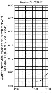
FREE AREA VELOCITY (FT/MIN) Based on STANDARD AIR- .075 lb. per cubic foot. Ratings do not include the effects of screen. 15 minute test duration
