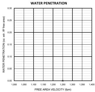
The AMCA Water Penetration Test provides a method for comparing various louver models and designs as to their efficiency in resisting the penetration of rainfall under specific laboratory test conditions. The point of zero water penetration is defined as that velocity where the water penetration curve projects through .01 oz of water penetration per sq. ft. of louver area. The beginning point of water penetration for RSR-900HP is 1250 fpm free area velocity.
