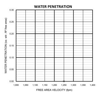
The AMCA Water Penetration Test provides a method for comparing various louver models and designs as to their efficiency in resisting the penetration of rainfall under specific laboratory test conditions. The point of zero water penetration is defined as that velocity where the water penetration curve projects through .01 oz of water penetration per sq. ft. of louver area. The beginning point of water penetration for RSR-545V is 1250 fpm free area
