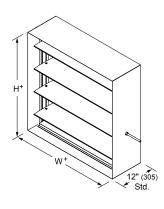
Sleeve (optional) <sup>+</sup>Damper dimensions furnished approximately 1/4" (6) undersize (sleeve thickness not included.
