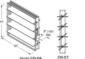
Model CD-58 (standard) \*Damper dimensions furnished approximately 1/4" (6) undersize (Drive axle supplied loose for field installation)
