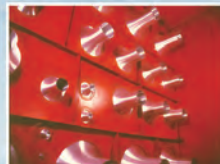
流量噴嘴 Multiple Nozzles for Flow Measurement
