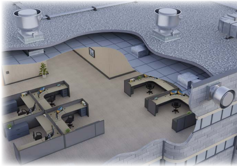
General HVAC Roof & Wall Exhaust
