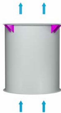
VUO Vertical Discharge Up, Ceiling Hung Support Brackets On Outlet
