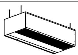
For tandem mounted units, center support required. The (2) center mounting holes are centerline of unit and 7.5/8" from front and rear of unit.
