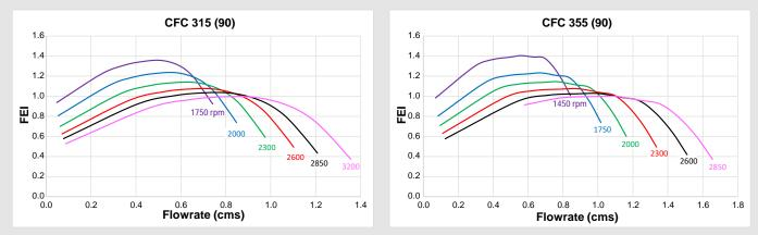
Performance certified is for installation type D - Ducted inlet, Ducted outlet. Power rating (kW) does not include transmission losses. Performance ratings do not include the effects of appurtenances (belt cover). FEI<sub>T</sub> values are calculated in accordance with ANSI/AMCA Standard 208 and are based on default motor efficiencies (Belt Driven type). FEI<sub>T</sub> values for fans with specific motors will vary slightly from those shown. Fan speed shown in RPM.
