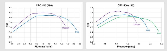
Performance certified is for installation type D - Ducted inlet, Ducted outlet. Power rating (kW) does not include transmission losses. Performance ratings do not include the effects of appurtenances (accessories). FEI<sub>T</sub> values are calculated in accordance with ANSI/AMCA Standard 208 and are based on default motor efficiencies (Direct Driven type). FEI<sub>T</sub> values for fans with specific motors will vary slightly from those shown. Fan speed shown in RPM.
