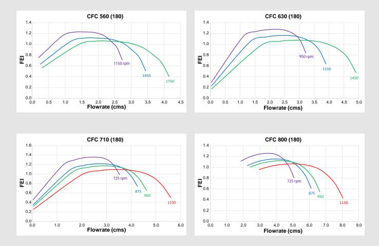
Performance certified is for installation type D - Ducted inlet, Ducted outlet. Power rating (kW) does not include transmission losses. Performance ratings do not include the effects of appurtenances (accessories). FEI<sub>T</sub> values are calculated in accordance with ANSI/AMCA Standard 208 and are based on default motor efficiencies (Direct Driven type). FEI<sub>T</sub> values for fans with specific motors will vary slightly from those shown. Fan speed shown in RPM.
