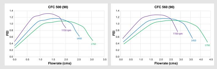
Performance certified is for installation type D - Ducted inlet, Ducted outlet. Power rating (kW) does not include transmission losses. Performance ratings do not include the effects of appurtenances (accessories). FEI<sub>T</sub> values are calculated in accordance with ANSI/AMCA Standard 208 and are based on default motor efficiencies (Direct Driven type). FEI<sub>T</sub> values for fans with specific motors will vary slightly from those shown. Fan speed shown in RPM.
