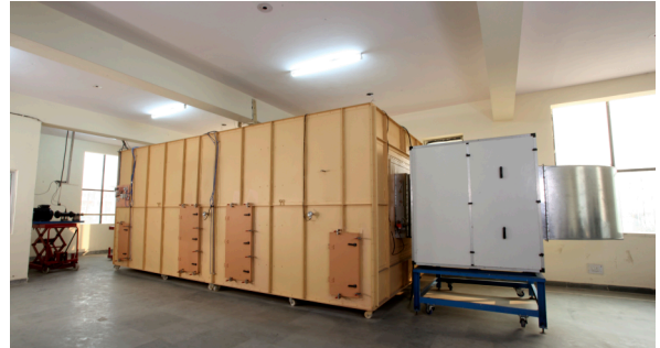
Blowtech's Fan Test Lab as per AMCA210
