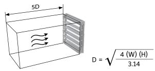
AMCA Figure 5.2 was established to represent a ducted damper that is exhausting into an open area. In this configuration entrance losses are minimized by a straight duct run upstream of the damper.
