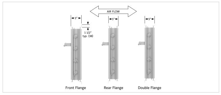
**Ruskin TED50DC** is rated for airflow in either direction, but Ruskin defines the "front" of the damper as the opposite side of the jackshaft and the "rear" as the jackshaft side. Unless specifically ordered otherwise, when looking at the concealed linkage side of the damper and the bottom blade turns clockwise to open, then the "front" surface is adjacent on the right.
