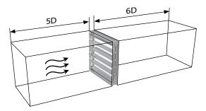
AMCA Figure 5.3 was established to represent a fully ducted damper with straight duct upstream and downstream. With entrance and exit losses minimized by this straight duct arrangement, this configuration has the lowest pressure drop of all three configurations.
