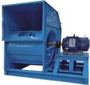
GUMSUNG POONG RYUK Co.,Ltd certifies that the GOA-DS Fan series shown herein is licensed to bear the AMCA Seal. The ratings shown are based on tests and procedures performance with accordance with AMCA publication 211.
