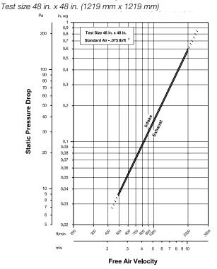
Model K6746HP resistance to airflow (pressure drop) varies depending on louver application (air intake or air exhaust). Free area velocities (shown) are higher than average velocity through the overall louver size. See louver selection information. (Test Figure 5.5-6.5)
