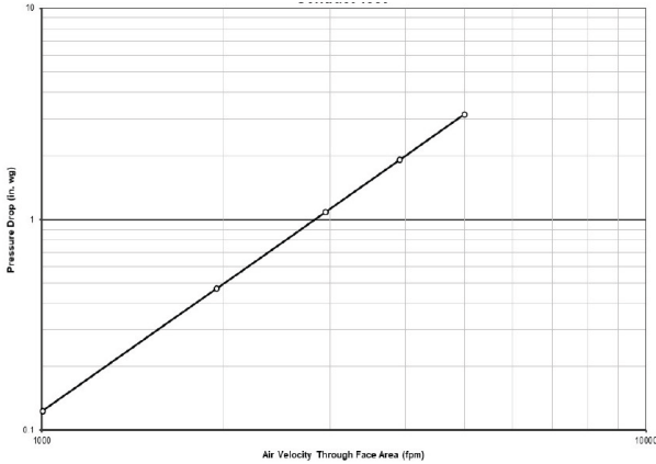
The maximum static pressure drop for specified air flow at standard air density
