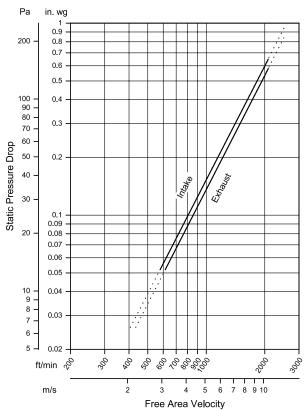
Model K6746MDE resistance to airflow (pressure drop) varies depending on louver application (air intake or air exhaust). Free area velocities (shown) are higher than average velocity through the overall louver size. See louver selection information. (Test Figure 5.5-6.5)
