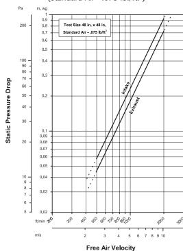
Louver Type SCH201 resistance to airflow varies depending on louver application (air intake or air exhaust). Free area velocities (shown) are higher than the average velocity through the overall louver size. (Test Figure 5.5-6.5)
