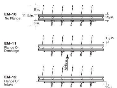
The APC allows field setting of relief pressure on all EM dampers. If more than a single section, a APC will be required for each section. Maximum pressure set limitations are as follows:
