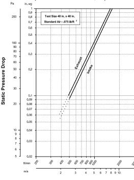
Louver Type SCC550MD resistance to airflow varies depending on louver application (air intake or air exhaust). Free area velocities (shown) are higher than the average velocity through the overall louver size. (Test Figure 5.5-6.5)
