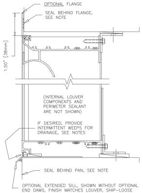
NOTE: SEALANT, BACKER ROD, NON-COMPRESSIBLE DEAD-LOAD SHIMS, SEPARATION OF DISSIMILAR MATERIALS AND SUBSTRATE ARE NOT BY LOUVER MANUFACTURER, SHIM AS NEEDED, PERIMETER SEALANT REQUIRED TO PASS ANSI/AMCA 550 HIGH VELOCITY WIND DRIVEN RAIN.
