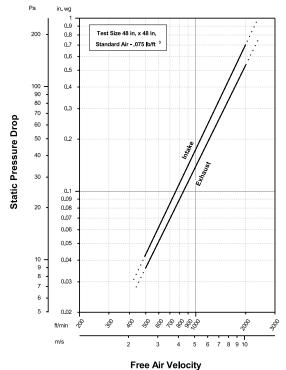
Model EVH-302D resistance to airflow (pressure drop) varies depending on louver application (air intake or air exhaust). Free area velocities (shown) are higher than average velocity through the overall louver size. See louver selection information. (Test Figure 5.5-6.5)
