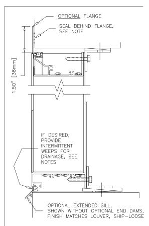
NOTE: SEALANT, BACKER ROD, NON-COMPRESSIBLE DEAD-LOAD SHIMS, SEPARATION OF DISSIMILAR MATERIALS AND SUBSTRATE ARE NOT BY LOUVER MANUFACTURER, SHIM AS NEEDED, PERIMETER SEALANT REQUIRED TO PASS ANSI/AMCA 550 HIGH VELOCITY WIND DRIVEN RAIN.
