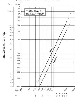
Free Air Velocity Louver Type K8206AMD resistance to airflow is shown with louver blades fully open. Resistance (pressure drop) varies depending on louver application (air intake or air exhaust). Free area velocities (shown) are higher than average velocity through the overall louver size.
